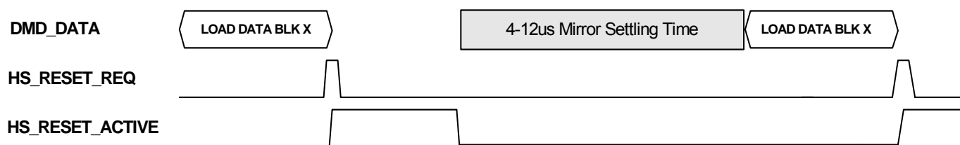
Figure 14 Typical Load and Reset Sequence on a single block with Mirror settling
